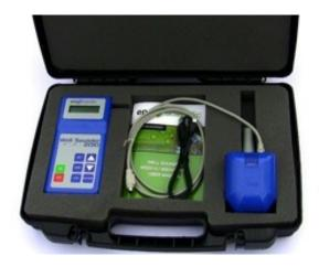
The Well Sounder 2010 PRO is a simple to use self-contained portable acoustic ranging instrument designed specifically to find the distance through a well casing or sounding tube to the water surface. However, it also can be used to measure any closed pipe, straight or crooked.
