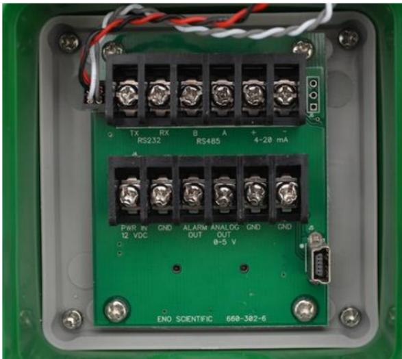
6 – Attach signal wiring.
