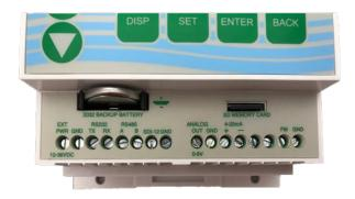
There are 3 available serial output options of which one can be software selected at a time. RS232, RS485 Modbus, and SDI-12.
