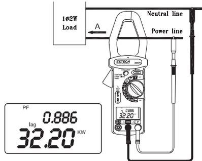
Note that **LEAD** and **LAG** icons are also displayed on the LCD to inform the user that the voltage is leading or lagging the current with regard to phase.
