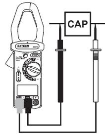
**Note:** Large valued capacitors will take a long period of time to charge and to auto-range to the correct range. (up to 60 seconds in the worst case). For improved resolution and shortest test time, manually pre-selecting the proper range is recommended.
