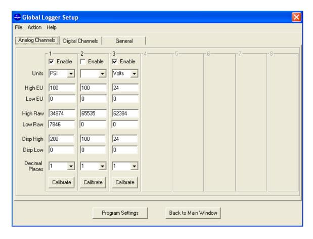
The PL200H Logger comes factory calibrated but you may want to re-calibrate on occasion. The pressure sensor is designed to measure over the range of 0-200 psi but it can be calibrated at lower pressures. The screen above shows channel one calibrated at 100 psi but set to display up to 200 psi on the main screen.
