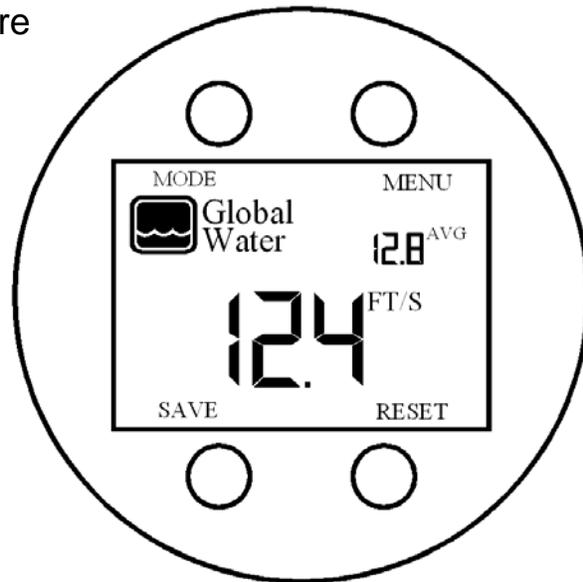
The MENU button is used to view stored data, delete data, set the flow units to FT/S or M/S, and change the calibration setting. Press the MENU button for 2 seconds to enter the setup menu. In menu mode, the labeling of the 4 buttons on the LCD display may change to indicate different functions.
