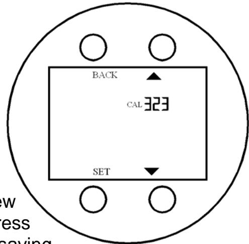
The calibration factor is equal to the rotation speed of the propeller in revolutions per minute that is equivalent to 1 foot per second of water velocity. It is used to scale the rotation of the propeller to the water velocity in FT/S. In the example shown, 323 RPM = 1 FT/S. The calibration factor must be set in the range of 200-400.
