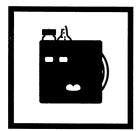
**5.** Shake the ampul again and place the ampul in the right top opening of the color comparator.
