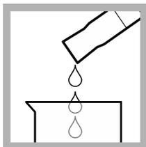
**2.** Pour 25 mL of the standard solution into a 50-mL plastic beaker.
