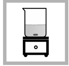
4. Add a stir bar to the first standard solution. Put the standard solution on an electromagnetic stirrer. Stir at a moderate rate.
