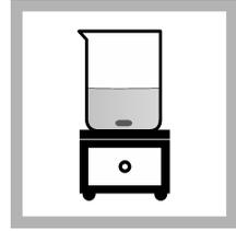
4. Add a stir bar. Put the beaker on an electromagnetic stirrer. Stir at a moderate rate.
