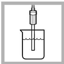
5. Put the probe in the sample with the sensor fully in the sample. Do not put the probe on the bottom or sides of the beaker.
