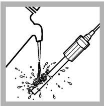
5. Rinse the probe with deionized water. Dry the probe with a lint-free cloth.
