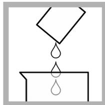
**3.** Add one Ammonium Ionic Strength Adjustor (ISA) Solution Pillow to each 25 mL of standard solution.
