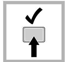
**8.** Stir for 30 to 60 seconds, then read the value of the standard solution. The meter accepts or rejects the result.
