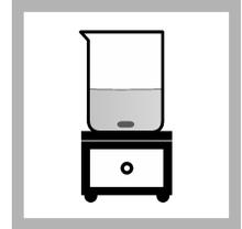
**4.** Add a stir bar. Put the beaker on an electromagnetic stirrer. Stir at a moderate rate.
