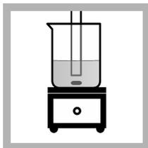
**6.** Put the probe in the standard solution with the sensor fully submerged. Do not put the probe on the bottom or sides of the beaker.
