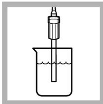
**6.** Put the probe in the standard solution with the sensor fully in the solution. Do not put the probe on the bottom or sides of the beaker.
