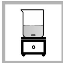
**4.** Add a stir bar to the first standard solution. Put the standard solution on an electromagnetic stirrer. Stir at a moderate rate.
