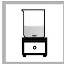
**3.** Add a stir bar. Put the beaker on an electromagnetic stirrer. Stir at a moderate rate.
