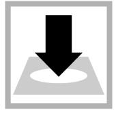
**14.** Insert the vial into the cell holder. DR 1900: Push **READ 2**.
