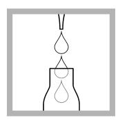
**11.** Carefully pipet into the same vial: **0.3 mL** of **solution C**.
