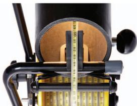
To test entire system, Hold the center pin on the probe against the stud on the back of the axle; touch the probe body against the screw on the frame. The buzzer will sound if the system is okay. **Make sure sensitivity dial is turned fully clockwise.**
