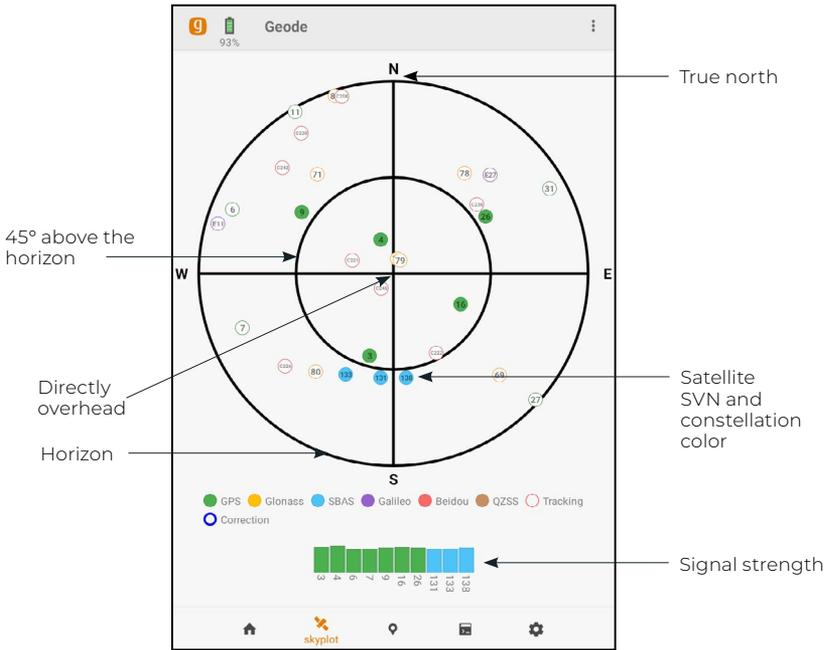
The Skyplot page is meant to be used as a guide. It shows the relative visibility of satellites in the sky, but it is not an absolute reference for satellites used in the positioning solution.
