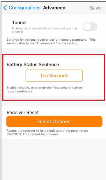
This gives the option to choose how frequently the Geode sends a battery status message. The message is used by Geode Connect and other applications to display the battery capacity status. The default setting is 10 seconds.
