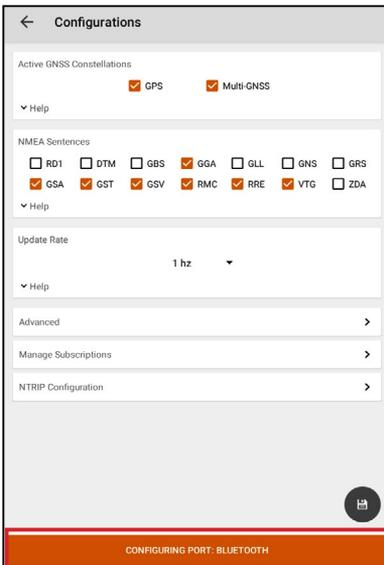
The Geode remembers its settings *per connection type*. You can use the Port Connection option to configure these settings for each connection type, without physically switching the connection for the Geode.
