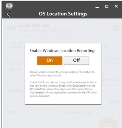
Select **On** to turn on Windows Location Services. Once the services are enabled, it is no longer necessary to keep Geode Connect open. If you choose to close Geode Connect, you will need to connect to the Geode via the third-party app or through Settings in Windows.
