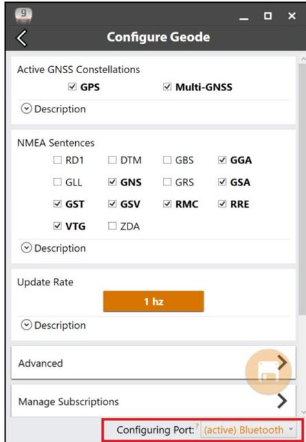
This affords you a certain amount of flexibility in the field. If you have multiple uses for the Geode and would prefer not to reconfigure it each time you switch tasks, the Geode can be configured per connection type for each specific task.
