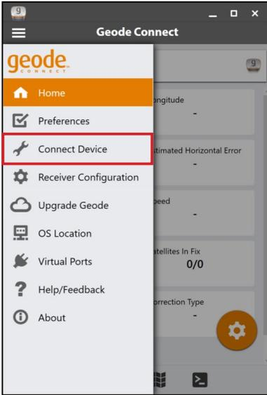
The Connect Device screen allows you to connect your Windows device to the Geode.
