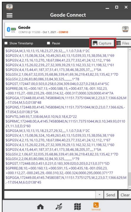
To stop recording, tap the timer that replaced the Capture button. The string of NMEA sentences will be saved.
