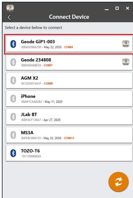
*Note: If your Geode doesn't show up in the list of devices, check to make sure it is turned on and not paired with another device. Then tap the refresh icon at the bottom of the list of devices
