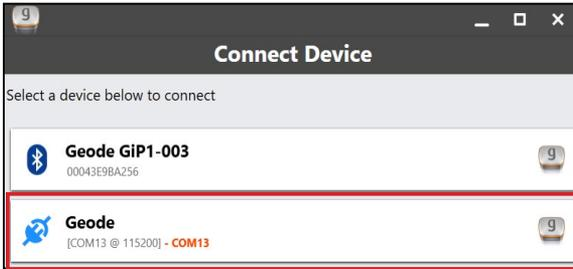
*Note: If your Geode doesn't show up in the list of devices, check to make sure it is turned on and not paired with another device. Then tap the refresh icon at the bottom of the list of devices
