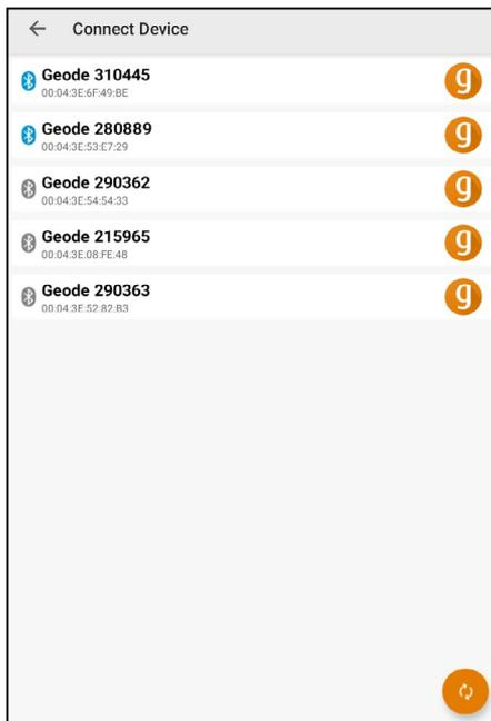
The app will display a list of local Bluetooth wireless devices. Identify your Geode via the serial number printed on its bottom panel.
