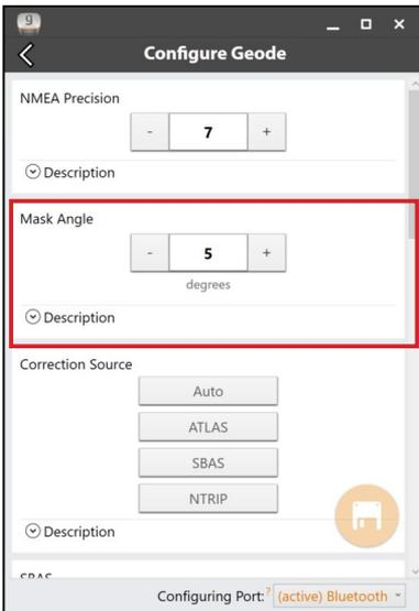
Specifies the elevation mask angle cutoff for the receiver. Any satellites below this angle will be ignored, even if available.
