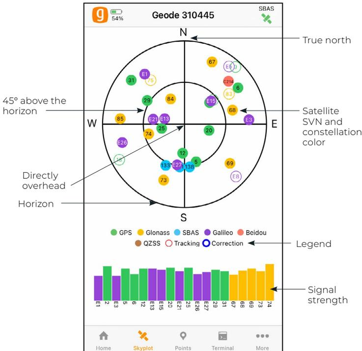
Satellite symbols outlined in red indicate that the satellites are being tracked, but they are not yet a part of the positioning solution. Satellite symbols outlined in blue indicate that a correction is being applied to the signal.
