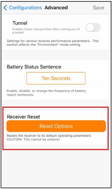
Reset Options allows you to select if you would like to perform a soft reset or a receiver reset.
