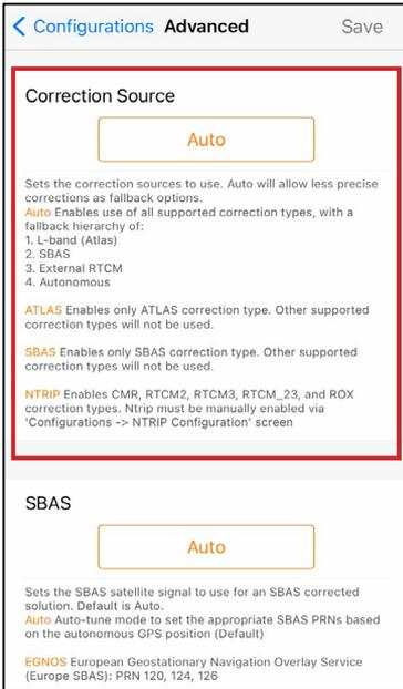
This specifies whether the Geode should automatically choose its correction source or accept only SBAS, NTRIP, or Atlas corrections. When the correction source is set to Auto, the Geode is programmed to choose a source according to accuracy level in the order of Atlas, SBAS, then NTRIP.
