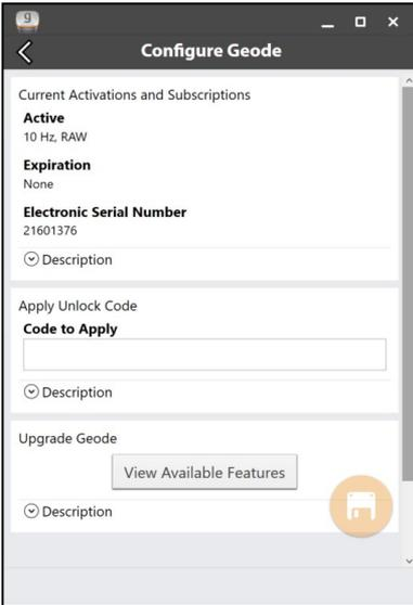
GNS3M devices offer a subscription to Atlas. This page allows you to view the details of your current subscription, apply the unlock code, and view the subscriptions that are available for activation.
