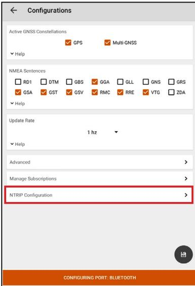
On the NTRIP Configuration screen you can set up NTRIP with your Geode. Enter the information supplied by your NTRIP service provider, including the caster IP address, port, username, and password.
