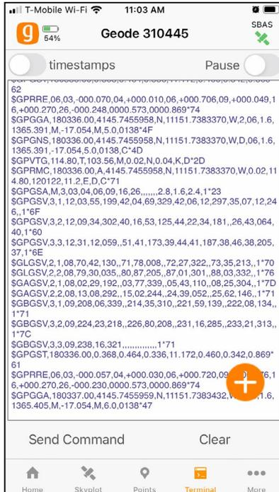
At the bottom of the Terminal page, you can send commands to the Geode. This gives you flexibility to configure the Geode and customize data output.
