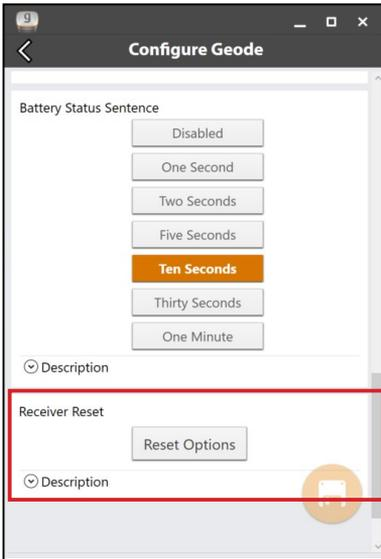
Reset Options allows you to select if you would like to perform a soft reset or a receiver reset.
