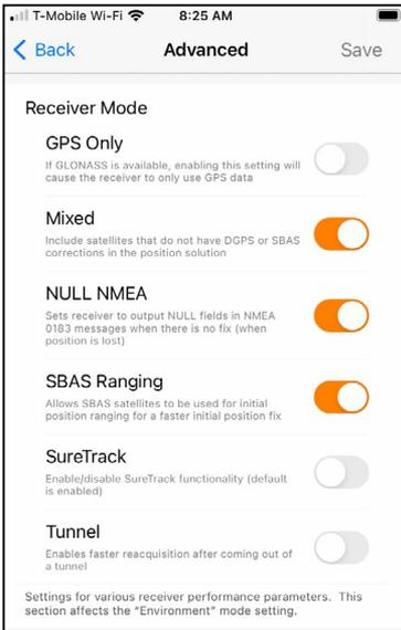
These options affect how the Geode collects and processes positioning information, as well as how it outputs certain types of data.
