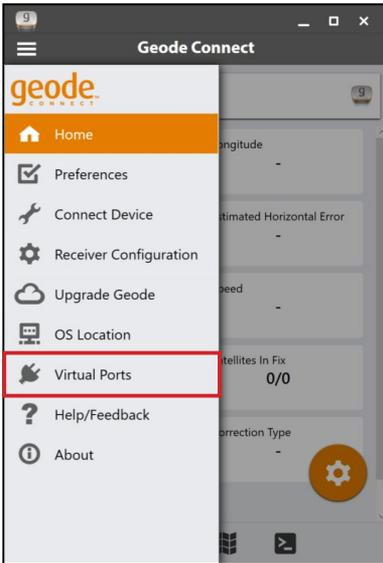
Geode Connect for Windows PC has a Virtual COM Port Driver. You can use this driver to configure virtual COM ports as writeable. Once writeable, these ports can be used for two-way communication between the Geode and third-party apps, allowing the apps to both receive and send information to the Geode.
