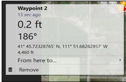
Geode Connect will show you the waypoint's distance and bearing compared to your current position. It will also display the latitude, longitude, and altitude of the waypoint.
