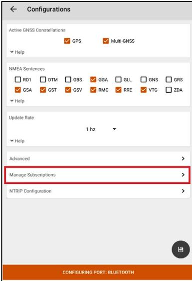
GNS3M devices offer subscriptions for Atlas. This screen allows you to view the details of your current subscription, apply unlock codes, and view the subscriptions that are available for activation.
