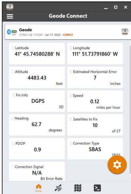
From the toolbar on the bottom of the page, you can access the Skyplot, Map, and Terminal pages. Tap on the receiver name at the top to change receivers. Tap on the Settings menu in the upper left corner to configure the currently connected receiver.
