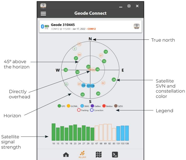
Satellite symbols outlined in red indicate that the satellites are being tracked, but they are not yet a part of the positioning solution. Satellite symbols outlined in blue indicate that a correction is being applied to the signal.
