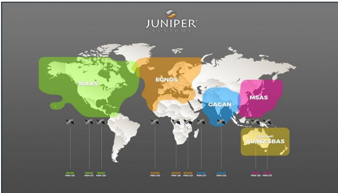
In areas of overlap, the best practice is to select a specific SBAS service from which the Geode should accept corrections data.
