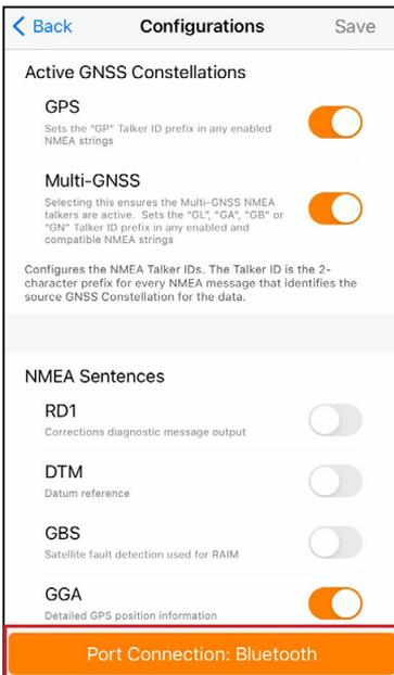
The Geode remembers its settings *per connection type*. You can use the Port Connection option to configure these settings for each connection type, without physically switching the connection for the Geode.
