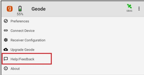
This feature links directly with the email account configured to the device and opens an email addressed to Juniper Systems Support. The email includes detailed configuration commands from the Geode. This allows Juniper Systems Support to diagnose and solve the problem more efficiently. This info is also used when purchasing a feature upgrade for the Geode.
