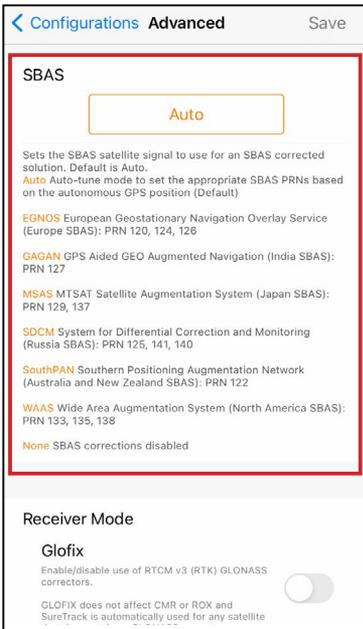
This specifies which SBAS satellites the Geode should use for GPS correction. Usually, selecting Auto is sufficient because the various SBAS services cover different geographical areas. However, there are some areas where these services overlap (see map below).
