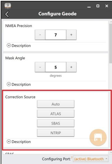
This specifies whether the Geode should automatically choose its correction source or accept only SBAS, NTRIP, or Atlas corrections. When the correction source is set to Auto, the Geode is programmed to choose a source according to accuracy level in the order of Atlas, SBAS, then NTRIP.
