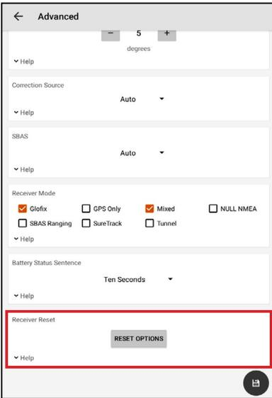
Reset Options allows you to select and perform a soft reset or a receiver reset.
