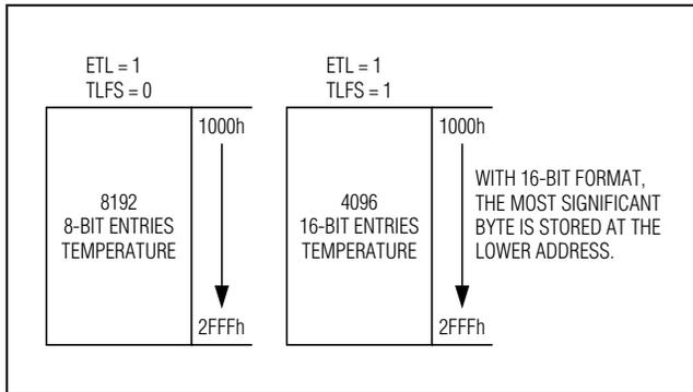
Figure 7. Temperature Logging
