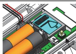
Open the mote door and install the rechargeable batteries. Press the button on the mote for 3 seconds.
