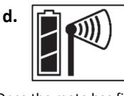
Once the mote has finished joining the network, the "x" icon is removed and the channel count on the station LCD increases by two (one for the sensor measurement and one for the mote battery).
