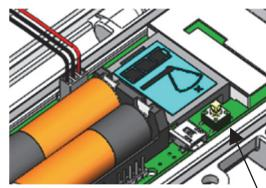
Open the mote door and Install the rechargeable batteries. Press this button on the mote for 3 seconds.
