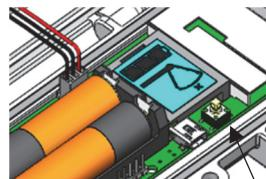
Open the mote door and install the rechargeable batteries. Press the button on the mote for 3 seconds.
