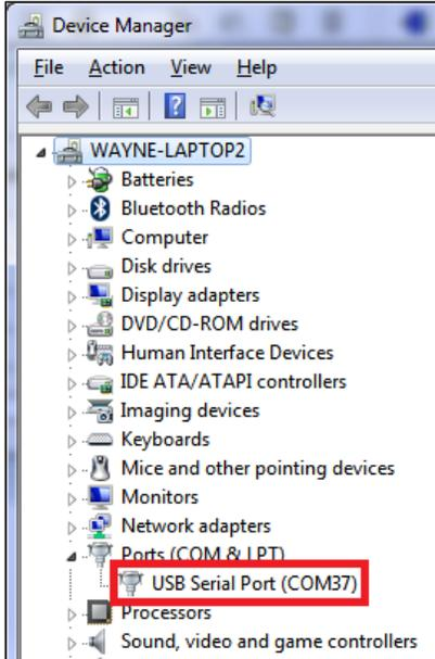
A shortcut to the device manager is provided in the File menu of RL-Loader™. The example on the left shows a RainLog™ connected on com port 37. A new number will be assigned for each USB port on the computer. New port numbers will also be generated if you have more than one RainLog. It is suggested that you use the same USB port each time as this makes it easier to track and RL-Loader™ will automatically try the last port number used.
