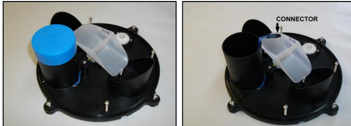
3. Connect the RainLog™ to the connector and place the RainLog™ inside the tube. Place the desiccant pack in the tube with the RainLog. Replace the blue cover.
