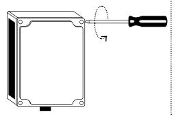
Install 6 AA alkaline batteries in the battery compartment.
