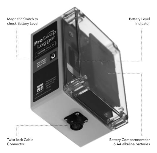
The Power Pack cover utilizes captive screws. Use a Phillips head screwdriver to loosen the 4 screws and remove the cover to access the battery compartment.
